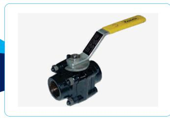
The Forged Steel Ball Valves are rugged in construction and are designed as per **BS 5351 (ISO 17292)** standards. The material of construction offered is **ASTM A105** Forged Steel. The trims can be supplied in **SS304** or in **SS316**.
